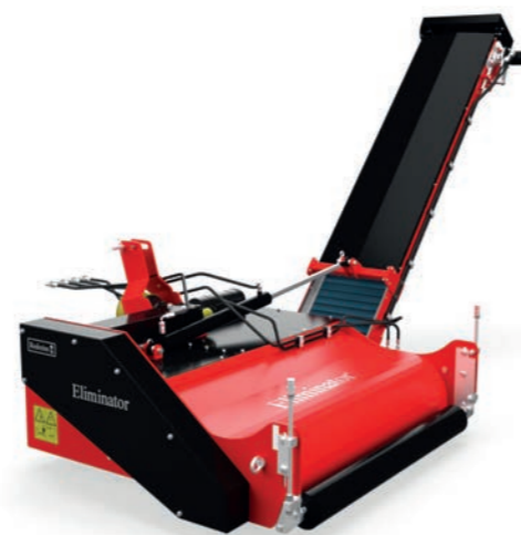
Adjustable conveyor speed to control the rate of material flow.
