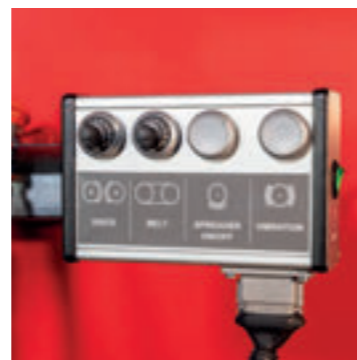
PotiPro control system allows for changes to spreading width and thickness on the move.
