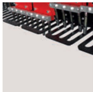
Turf fingers hold down grass to ensure no damage through pulling.
