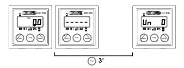
During the programming phase, you can use the "+" and "-" buttons to edit the value of the parameter, then press the "Prog" button to confirm your changes and move on to the next parameter;
