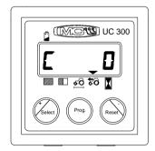
At this point, travel 100 metres (or 330 feet) in the machine and the number will increase automatically on the display. After covering this distance, press the "Prog" button to confirm the data. It is advisable to repeat this operation at least twice.
