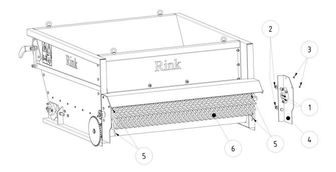
The brush roller (6) consists of 10 individual segments, which are interlinked. Both outer segments are secured on the shaft, each with three grub screws (5). To replace the brush roller proceed as follows:
